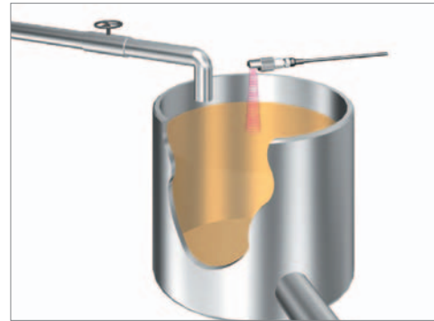
●Inspection of Solvent Tank Levels
