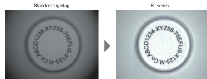
Faster lines make it necessary to increase shutter speeds, but then the clarity of workpiece images decreases.
